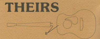
Dowel rod attachment. The only reinforcement between neck and body joint are some wooden dowels ("B"). This is cheaper than dove tailing, and also much weaker. Heel will often separate from body, due to pull of strings, or due to shock.
